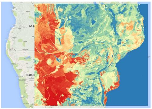
Figure 84: HiHydroSoil field capacity of the topsoil layer in the Southeast Africa database.
