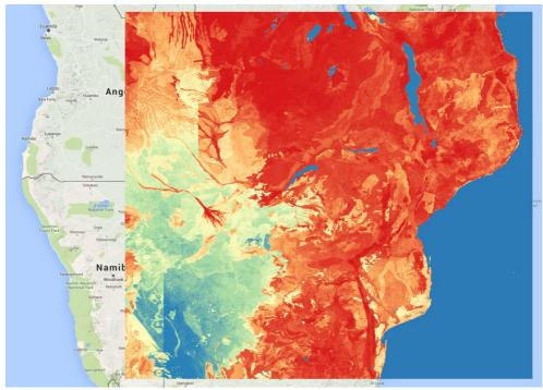
Figure 83: HiHydroSoil saturated conductivity of the topsoil layer in the Southeast Africa database.
